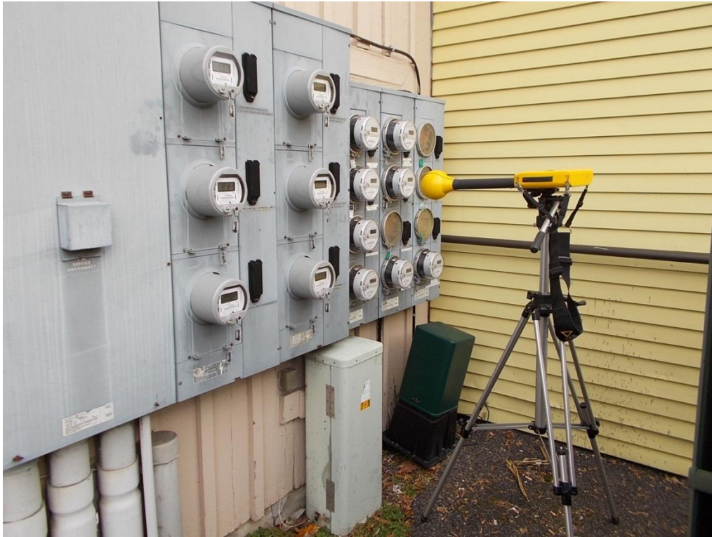
Figure 11. Use of the SRM-3006 to measure the duty cycle of smart meter emissions over a 30-minute period at a meter bank in Rutland.
