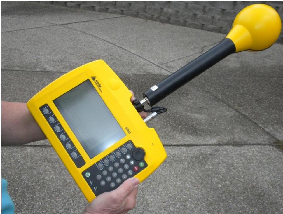
Figure 5. The Narda SRM-3006 Selective Radiation Meter is based on fast Fourier transform (FFT) spectrum analyzer technology and uses a probe/antenna to measure the absolute magnitude of incident RF fields across the frequency range of 26 MHz to 3,000 MHz and digitally converts the detected field to the equivalent percentage of the FCC MPE.
