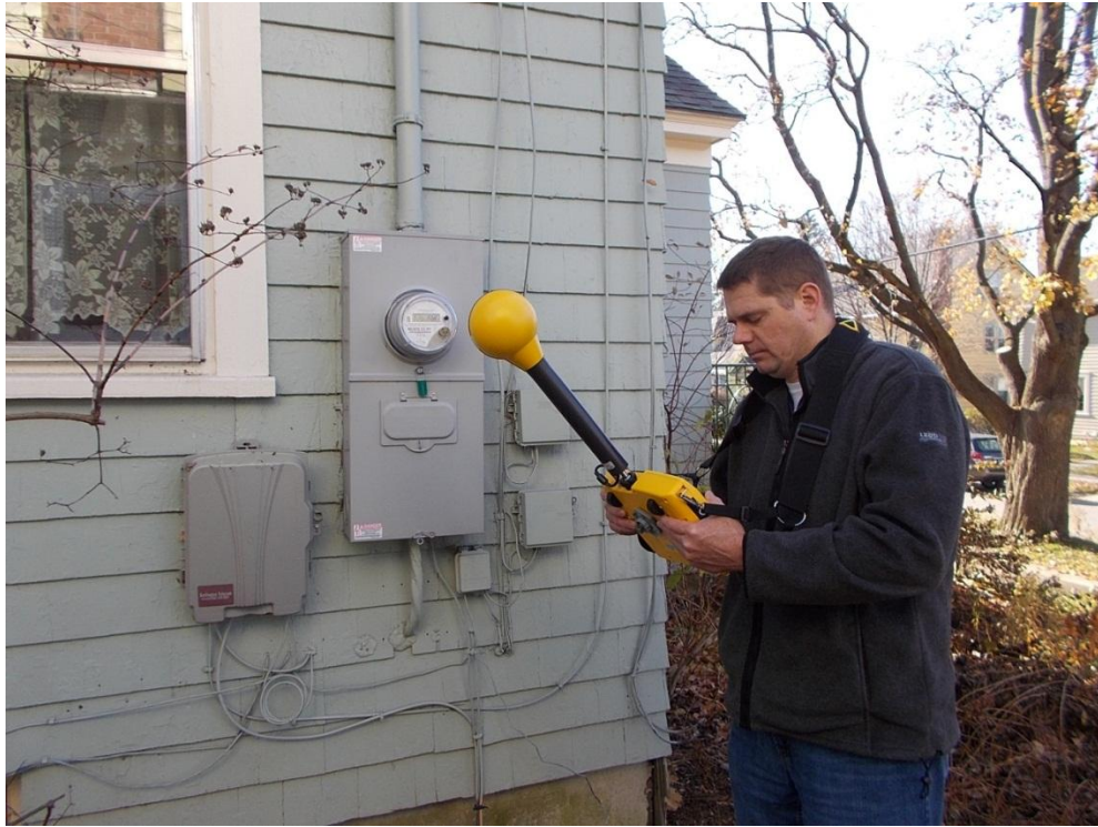
Figure 10. Measurement of RF fields in front of a residential smart meter installation. Measurements were made at distances from 1 foot to 10 feet in front of the meters.
